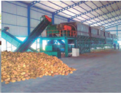
椰子抽絲烘乾打包機 Coconut Fiber Turn Key Plant ( with separating drying oven and automatic baler )
